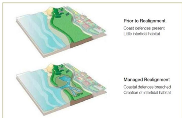
Figure 4: Managed realignment (ClimateTechWiki 2012)
